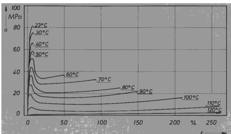
PLEXIGLAS® GS: Tensile strength  $\sigma$  ( \_\_\_\_\_ ), elongation at break  $\epsilon_R$  ( - - - - - ) and elastic modulus E ( - . - . - ) as a function of the temperature T
