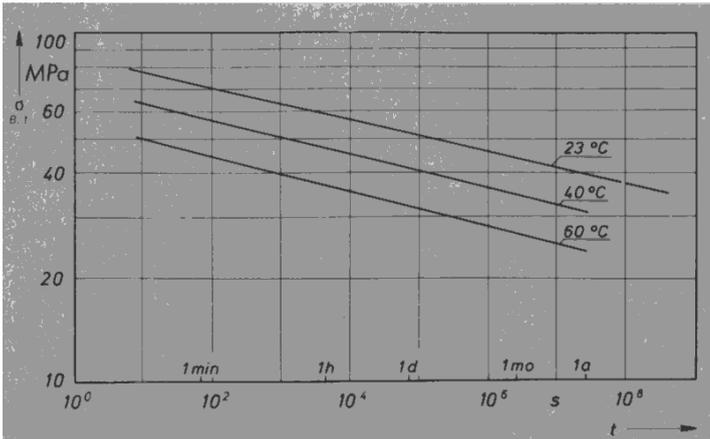
PLEXIGLAS® GS: Long-term tensile strength  $\sigma_{B,t}$  in water at increased temperatures: 23, 40 and 60 °C
